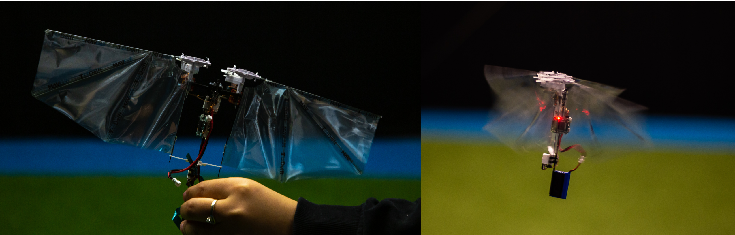
The DelFly Nimble is a highly mobile flying robot (drone), based on the characteristics of the fruit fly
